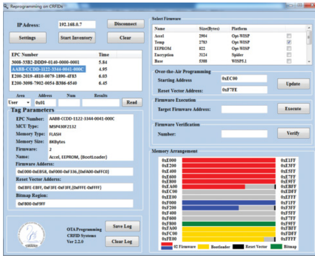
Fig. 10. User Interface passes encoded instructions through commercial RFID reader, receives the tag's reply and displays the results.
