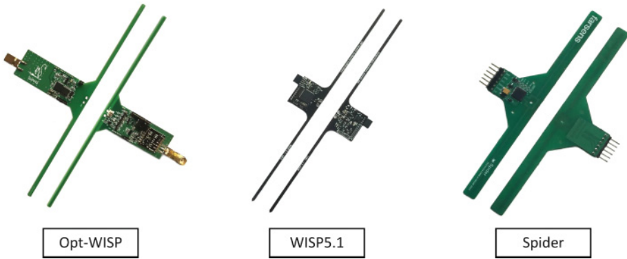
Fig. 1. Software-defined CRFIDs Opt-WISP and WISP5.1 and chip-based CRFID Spider.
